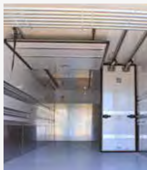
Drop down walls
